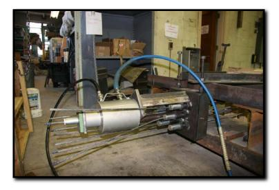
Post-tensioning with unbonded tendons (Sakai and Mahin 2003)
