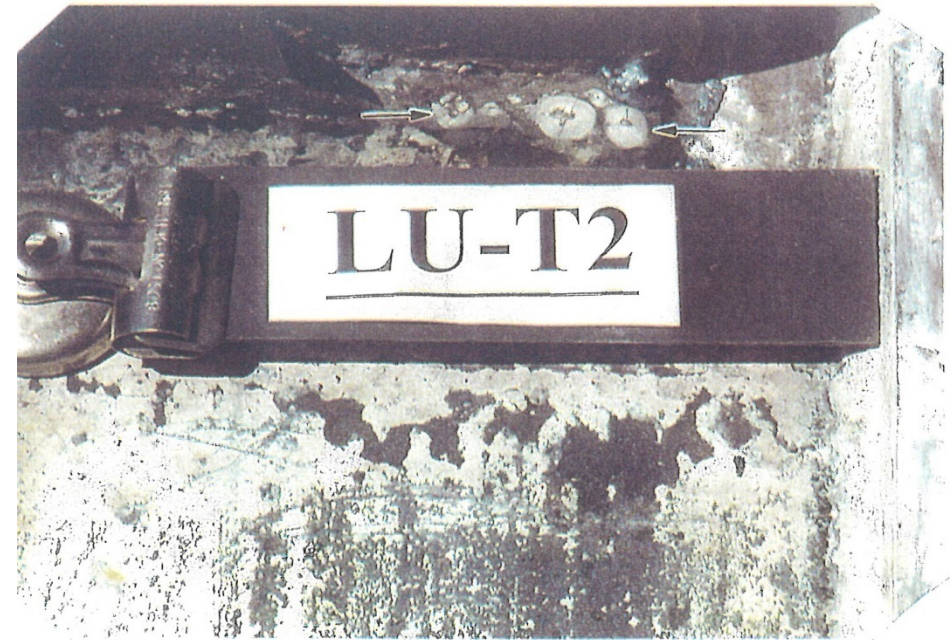
Figure 32. Examples of weld imperfections in Lehigh University connection LU-T2.
